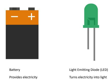
There's something special about the circuit element that we are using to produce light; it only makes light when electricity flows through it one way, but not the other. Remember positive and negative? Our special light is called a Light Emitting Diode (LED), and will turn only if they are placed in your circuit so that electricity flows from their positive leg to their negative leg. This means we have to pay special attention to how we place them in our circuit.
