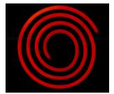
A heating coil – a special kind of resistor
